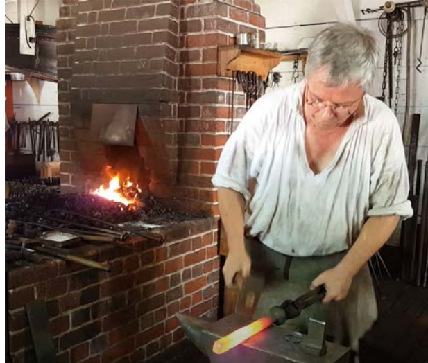
Master Blacksmith Ken Schwarz from Colonial Williamsburg's Anderson Armoury, forging the Market House Bell Clapper, June 22, 2015. https://www.youtube.com/watch?v=Y2gPg26PkrI
